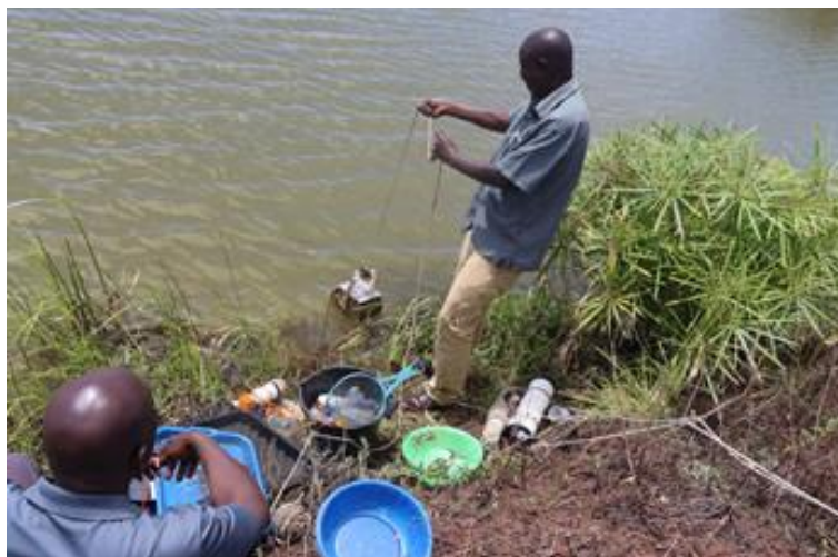
Plate 3: Deployment of the Ekman grab for sampling of macroinvertebrates at the bottom sediments in the Central Kenya region.
